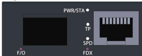
Fig. 2 WDM & SFP Front Panel of MCT-3512
