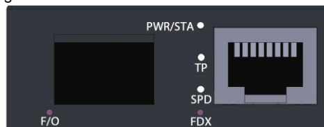
Fig. 2 WDM & SFP Front Panel of MCT-3002 Converter
