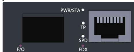
Fig. 2 WDM & SFP Front Panel of MCT-3002 Converter
