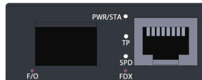
Fig. 2 WDM & SFP Front Panel of MCT-100 Converter
