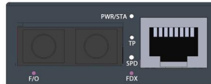
Fig. 1 Dual Fiber Front Panel of MCT-100 Converter
