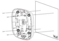
**Step 1.** Place the cable tray at the desired location and secure it with four self-tapping pointed screws. (Note: The diameter of each screw head should be between **4.4mm** and **8.8mm** to ensure firm mounting.)
