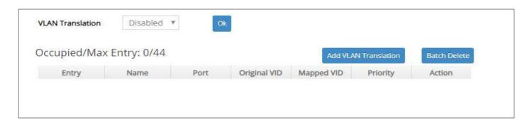
This table will display the overview of each configured VLAN mapping rule. Up to 44 VLAN mapping rules can be set up.
