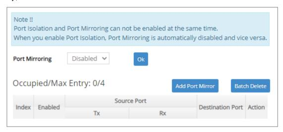
This table will display the overview of each configured port mirroring. Up to 4 sets of port mirroring can be set up.
