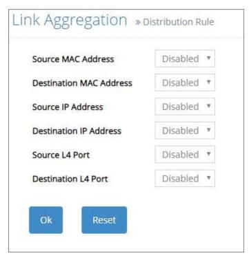
There are six rules offered for you to set up packets according to operations.
