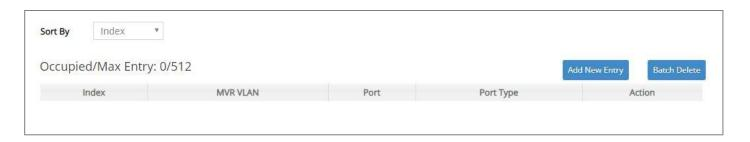
This table will display the overview of each configured MVR port entry. Up to 512 MVR port entries can be created.
