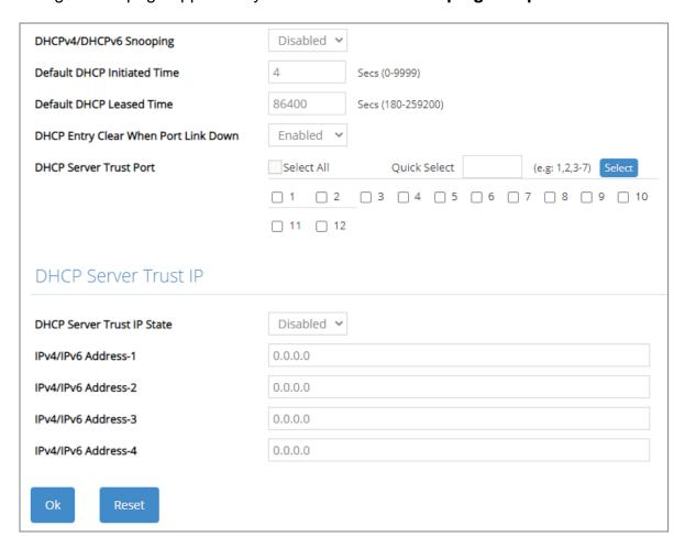
**DHCPv4/DHCPv6 Snooping:** Enable or disable DHCPv4/DHCPv6 Snooping function.
