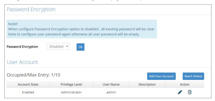
**Password Encryption:** Pull down the menu of **Password Encryption** to disable or enable MD5 (Message-Digest Algorithm). It is a widely used cryptographic hash function producing a 128-bit (16-byte) hash value, typically expressed in text format as a 32 digit hexadecimal number. Click **OK**, the new settings will be taken effect immediately. The default setting is disabled.
