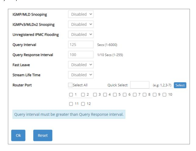
**IGMP/MLD Snooping:** When enabled, the Managed Switch will monitor network traffic and determine which hosts to receive multicast traffic.
