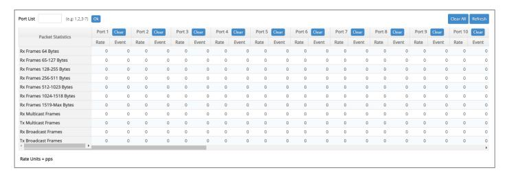
**Port List:** Enter the preferred port number (e.g.1, 2, 3-7) and then press the **OK** button, the port packet analysis statistics of the specified port(s) will be displayed immediately.
