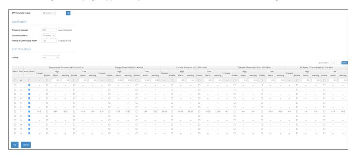
**SFP Threshold Enable:** Globally enable or disable the alarm notification of temperature/current/voltage/TX power/RX power for SFP ports of the Managed Swtich.
