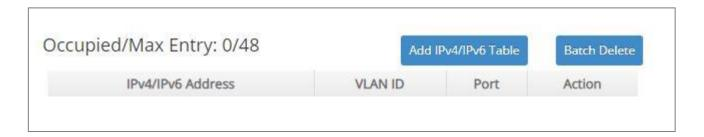
This table will display the overview of each configured static IPv4/IPv6 IP address and port mapping. Up to 48 static IP addresses can be created.
