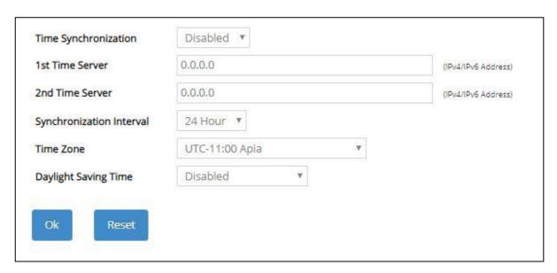
**Time Synchronization:** To enable or disable the time synchronization function.
