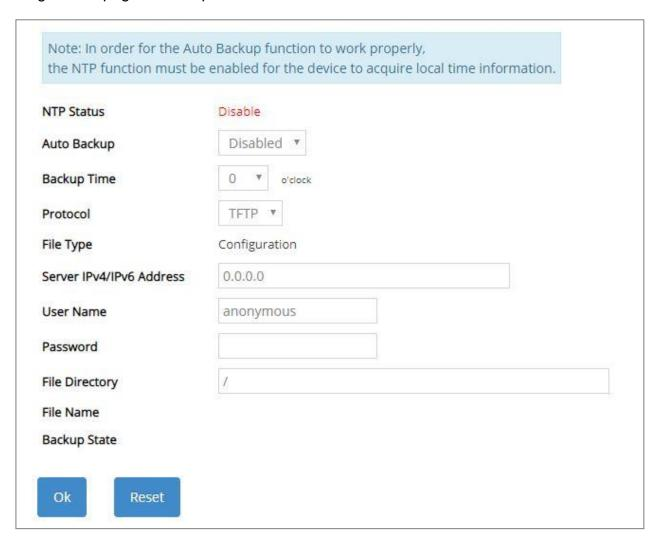
NTP Status: Display the current state of NTP server. Include Disable, Inactive and active 3 states.
