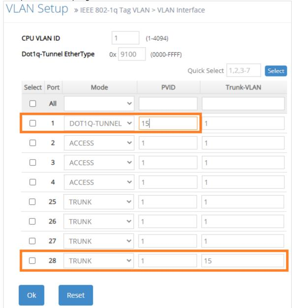
Check the VLAN status. Supposed that Port 1 carries dot1q-tunnel VLAN 15 while Port 28 trunk VLAN 15.
