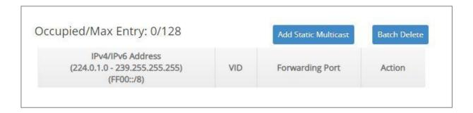
This table will display the overview of each configured static multicast entry. Up to 128 static multicast entries can be created.
