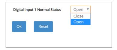
There is one Digital Input Normal Status option shown on the screen page. Normal Status refers to where the contact remains in one state unless actuated. The contact can either be normally open until closed by operation of the switch, or normally closed and opened by the switch action. You may choose either "Open" or "Close" as the normal status of electrical circuit by clicking this pull-down menu.
