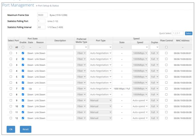
**Maximum Frame Size:** Specify the maximum frame size between 1518 and 9600 bytes. The default maximum frame size is 9600 bytes.
