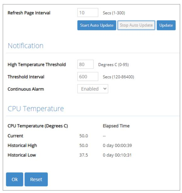
**Refresh Page Interval:** Automatically updates CPU temperature of the system at a specified interval in seconds. Please note that the value you assign in this parameter is temporarily used and will not be saved into the configuration file of the Managed Switch. This value will not be applied into the next system boot-up.
