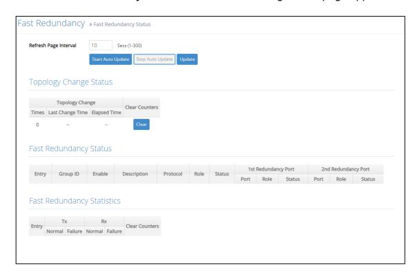
**Refresh Page Interval:** Automatically updates statistics of the Fast Redundancy Status page encompassing three main subdivisions at a specified interval in seconds. Please note that the value you assign in this parameter is temporarily used and will not be saved into the configuration file of the Managed Switch. This value will not be applied to the next system boot-up. Click **Start/Stop Auto Update** to activate auto-update; click **Update** to manually refresh the event log table once.
