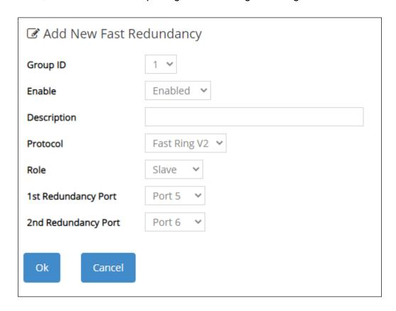
**NOTE:** To avoid the occurrence of loop, please do not connect Switch 1, 2, 3 & 4 together in the ring topology before the end of Fast Ring v2 configuration.
