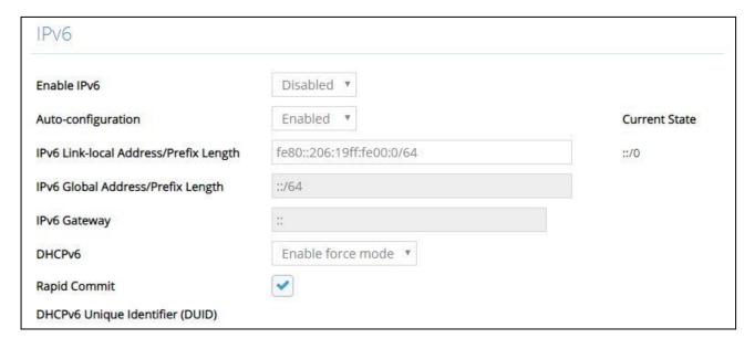
**Enable IPv6:** Click the checkbox in front of **enable IPv6** to enable IPv6 function on the Managed Switch.
