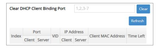
Clear DHCP Client Binding Port: Clear the DHCPv4/DHCPv6 snooping entry. Specify the DHCP client binding port, and click Clear to remove the intended DHCPv4/DHCPv6 snooping entry.
