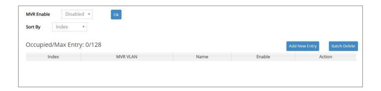
This table will display the overview of each configured multicast VLAN entry. Up to 128 MVR entries can be created.
