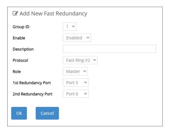
Step 2: Set up the Fast Ring v2 configuration on Switch 2, 3 & 4.
