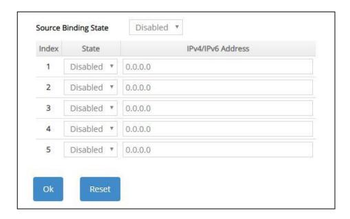
**Source Binding State:** Globally enable or disable IP source binding.
