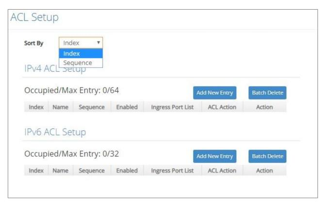
The IPv4 or IPv6 ACL tables will display the overview of each configured IPv4 or IPv6 ACL entry respectively. Up to 64 IPv4 ACL entries and 32 IPv6 ACL entries can be created.
