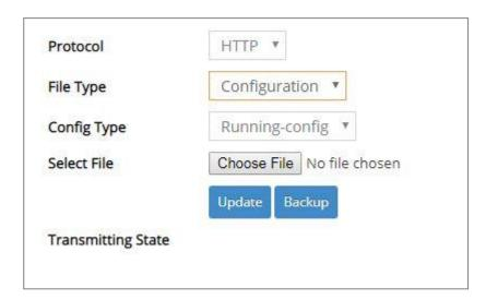
**Config Type:** There are three types of the configuration file: Running-config, Default-config and Start-up-config.
