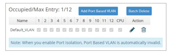
Since source addresses of the packets are listed in MAC address table of specific VLAN (except broadcast/multicast packets), in every VLAN the traffic between two ports will be two-way without restrictions.
