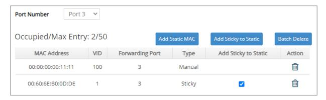
**NOTE:** The Managed Switch only supports port-based MAC security and does not support switch-based MAC security. The Managed Switch can support up to 50 entries of MAC security list per port.
