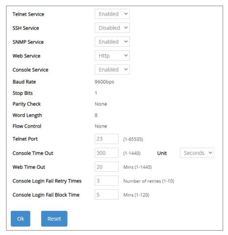
**Telnet Service:** To enable or disable the Telnet Management service.
