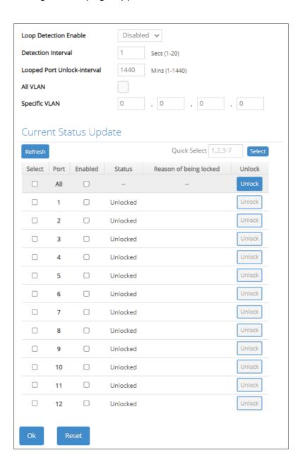
**Loop Detection Enable:** Enable or disable the Loop Detection function on a system basis. The default setting is disabled.
