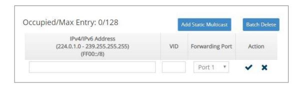
IPv4/IPv6 Address: Specify the multicast stream source IPv4/IPv6 address.
