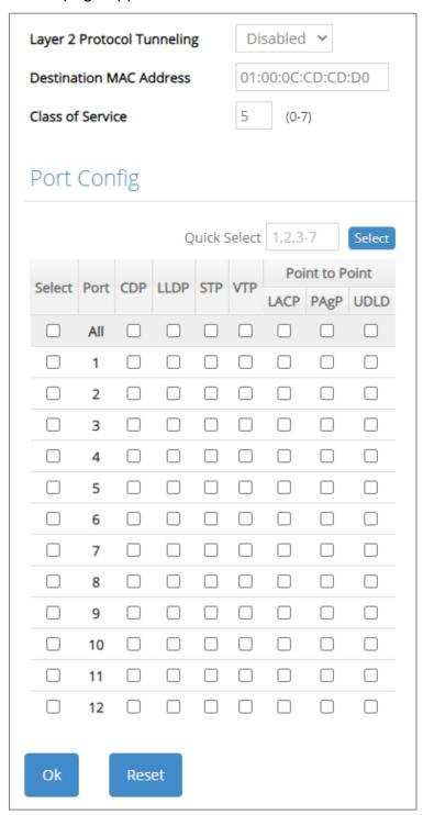
Layer 2 Protocol Tunneling: Enable or disable the Layer 2 Protocol Tunneling fuction globally.
