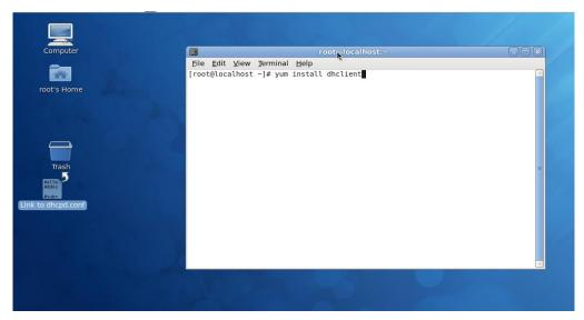
Linux Fedora 12 supports "yum" function by default. First of all, update DHCP client function by issuing "yum install dhclient" command.
