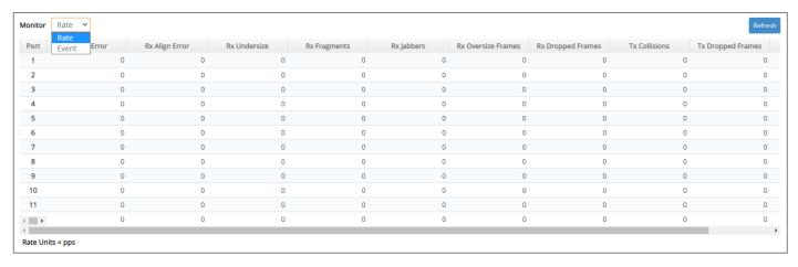
**Monitor:** Choose the way of representing the Port Packet Error Statistics from the pull-down menu. Either "Rate" or "Event" option can be chosen.
