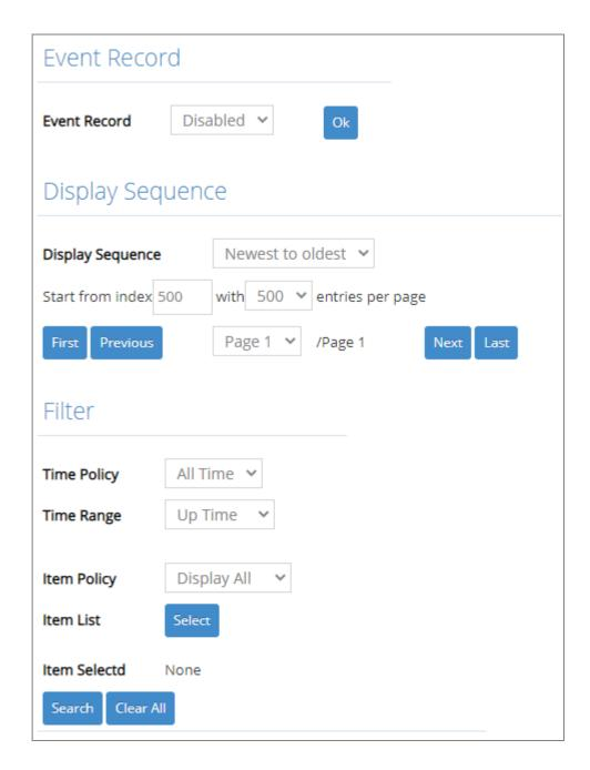
**Event Record:** Configure the Event Record function. Once it's **enabled**, the Managed Switch will fully preserve the entire event log after reboot, while the Managed Switch will erase the entire event log if Event Record is **disabled**. Click **OK** when you have finished the configuration.
