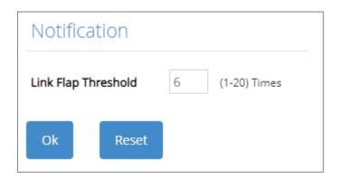
**Link Flap Threshold:** To configure the maximum time of each port's port link flap for sending the alarm trap and the syslog message. For example, if the threshold is configured as "3", it means that the Managed Switch will send the alarm trap and the syslog message out to the specified SNMP server and log server respectively when one port links down or links up 3 times. Valid range: 1~20 times. Default is 6 times.
