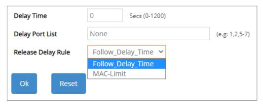
**Delay Time:** Specify the desired time the designated delay port(s) will delay to be activated. Valid range: 0~1200 seconds. Default setting is "0". "0" indicates "Disabled".
