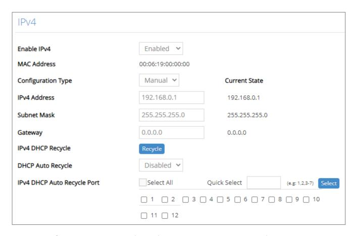
**Enable IPv4:** Click the checkbox in front of **enable IPv4** to enable IPv4 function on the Managed Switch.
