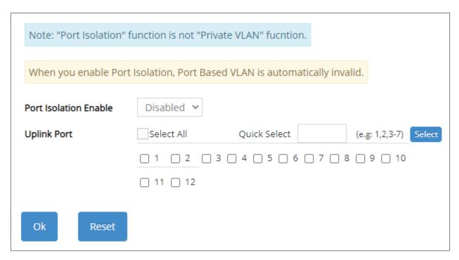
**Port Isolation Enable:** Enable or disable port isolation function. If port isolation is set to enabled, the ports cannot communicate with each other.
