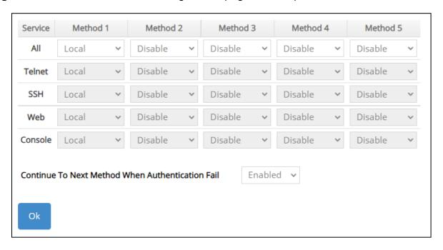
**Service:** The interfaces via which the user accesses the Managed Switch, including **All**, **Telnet**, **SSH**, **Web**, and **Console**.
