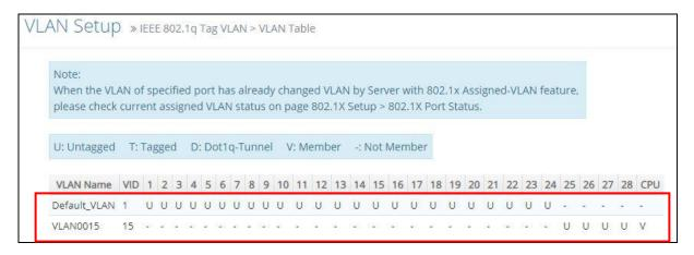
2. Now, change the Management VLAN 15 into VLAN 20 and includes Port 25, 26 and 27 under Access mode (It's necessary to include Port 26 to prevent the disconnection.)
