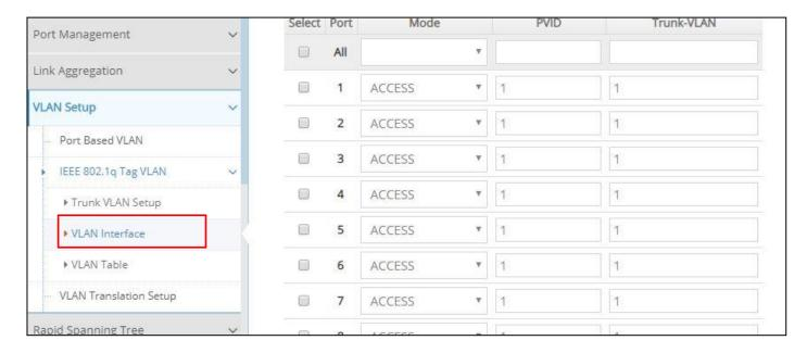
2. Create a new Data VLAN 11 that includes Port 1 and Port 28 as members. VLAN Setup>IEEE 802.1q Tag VLAN>VLAN Interface
