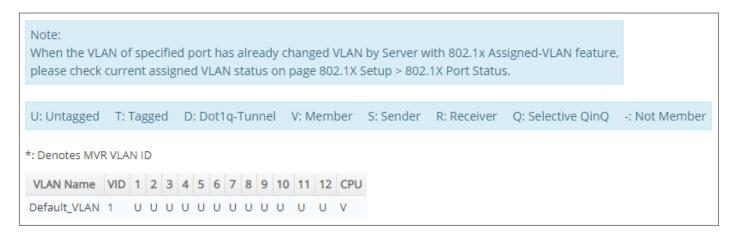
**VLAN Name:** View-only field that shows the VLAN name. If the VLAN name belongs to an "Enabled" multicast VLAN ID, it will be automatically changed into the one same as MVR name configured in **MVR > MVR System Setup** function.
