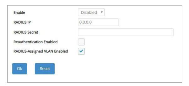
**Enable:** Enable or disable IEEE 802.1X/MAB on the Managed Switch. When enabled, the Managed Switch acts as a proxy between the 802.1X-enabled client and the authentication server. In other words, the Managed Switch requests identifying information from the client, verifies that information with the authentication server, and relays the response to the client.
