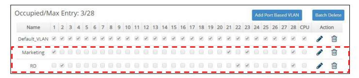
**NOTE:** By default, all ports are member ports of the Default\_VLAN. Before removing the Deafult\_VLAN from the VLAN table, make sure you have correct management VLAN and VLAN mode configurations, otherwise, incorrect configurations may disconnect your management PC to the Managed Switch immediately when you enter the command.
