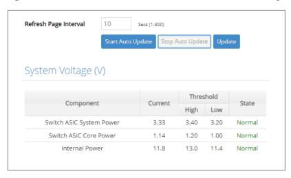
**Refresh Page Interval:** Automatically updates statistics and state of Managed Switch's ASIC system power, ASIC core power and internal power at a specified interval in seconds. Please note that the value you assign in this parameter is temporarily used and will not be saved into the configuration file of the Managed Switch. This value will not be applied into the next system bootup.
