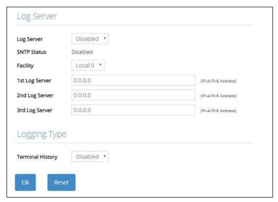
When DHCP snooping filters unauthorized DHCP packets on the network, the mal-attempt log will allow the Managed Switch to send event notification message to log server.
