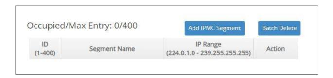
This table will display the overview of each configured IPMC segment. Up to 400 IPMC segments can be created.
