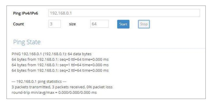
Enter the IPv4/IPv6 address of the host you would like to ping. You can also specify the count and size of the Ping packets. Click **Start** to start the Ping process or **Stop** to pause this Ping process.
