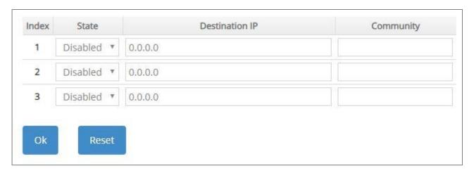
State: Enable or disable the function of sending trap to the specified destination.
