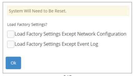
**Load Factory Settings Except Network Configuration:** It will set all the configurations of the Managed Switch back to the factory default settings. However, IP and Gateway addresses will not restore to the factory default. It is very useful when network administrators need to re-configure the system "REMOTELY" because conventional Factory Reset will bring network settings back to default and lose all network connections.
