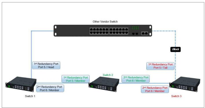
Fig. 4-2 Chain Example Diagram
