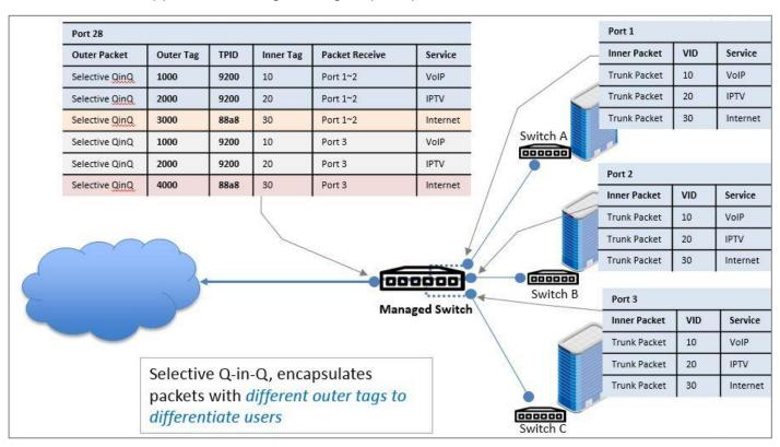
As the above figure shows, three clients are assigned three VLANs that the tag values are 10, 20 & 30 in Internet service. VLAN 10 corresponds to VoIP, VLAN 20 corresponds to IPTV and VLAN 30 corresponds to Internet. After the downlink ports enable Selective Q-in-Q function that connects Managed Switch to switch A, B & C, the packets will be packed with different external tags according to VLAN ID of service.
