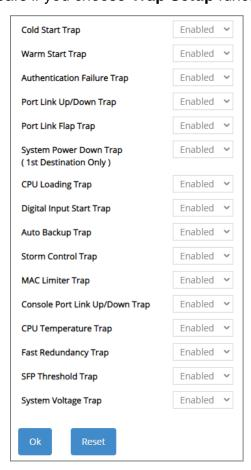
**Cold Start Trap:** Enable or disable the Managed Switch to send a trap when the Managed Switch is turned on.
