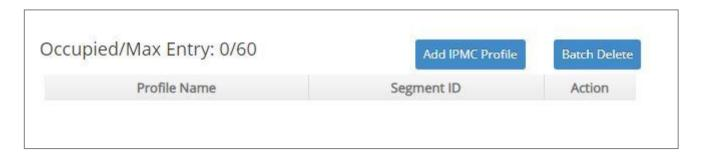
This table will display the overview of each configured IPMC profile. Up to 60 IPMC profiles can be registered.
