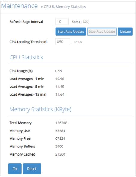
**Refresh Page Interval:** Automatically updates statistics of CPU & Memory at a specified interval in seconds. Please note that the value you assign in this parameter is temporarily used and will not be saved into the configuration file of the Managed Switch. This value will not be applied into the next system boot-up.
