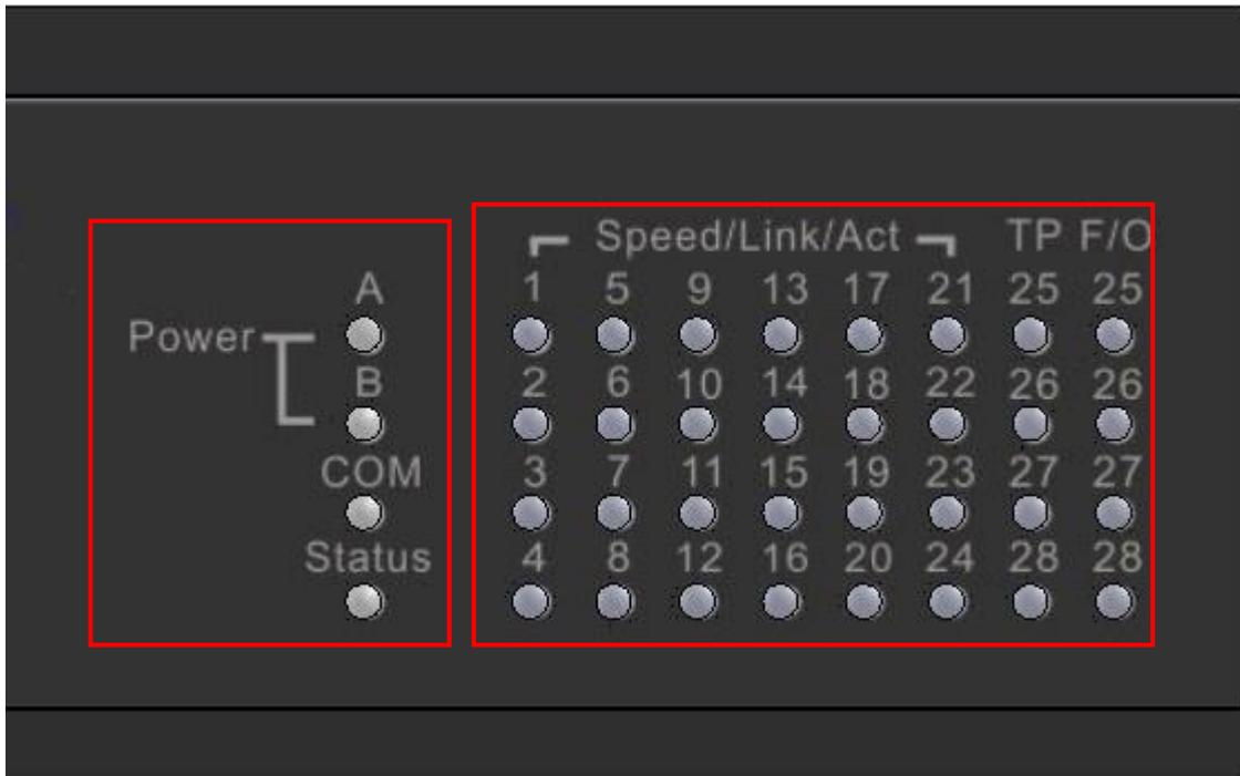
Figure 1-3. LEDs of FOS-3128 Managed Switch
