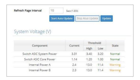
**Refresh Page Interval:** Automatically updates statistics and state of Managed Switch's ASIC system power, ASIC core power and Power A & B at a specified interval in seconds. Please note that the value you assign in this parameter is temporarily used and will not be saved into the configuration file of the Managed Switch. This value will not be applied into the next system bootup.
