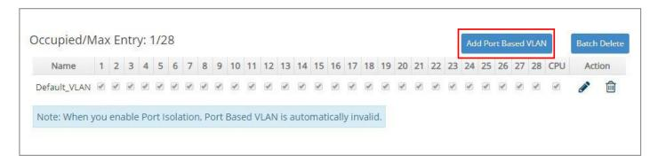
3. Add Port 1, 21, 23 and 28 in a group and name it to "Marketing". VLAN Setup>Port Based VLAN>Add Port Based VLAN
