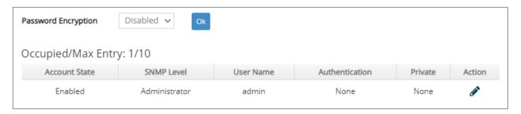
**Password Encryption:** Pull down the menu of **Password Encryption** to select one method to secure the password against potential malicious attacks.
