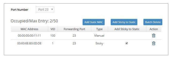
**NOTE:** The Managed Switch only supports port-based MAC security and does not support switch-based MAC security. The Managed Switch can support up to 50 entries of MAC security list per port.
