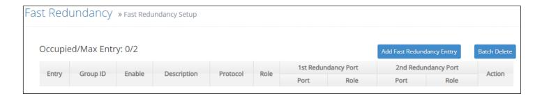
**1-3.** Please refer to each column parameter below, set "Group ID" = 1, "Enable" = Enabled, "Protocol" = Chain, "1st Redundancy Port" = Port 5, "1st Redundancy Port / Role" = Head, & "2nd Redundancy Port" = Port 6, click **OK** when completing the chain configuration for Switch 1.
