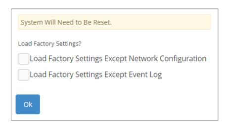
**Load Factory Settings Except Network Configuration:** It will set all the configurations of the Managed Switch back to the factory default settings. However, IP and Gateway addresses will not restore to the factory default. It is very useful when network administrators need to re-configure the system "REMOTELY" because conventional Factory Reset will bring network settings back to default and lose all network connections.
