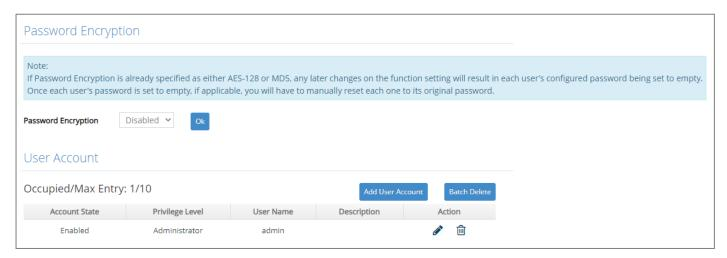
**Password Encryption:** Pull down the menu of **Password Encryption** to select one method to secure the password against potential malicious attacks.
