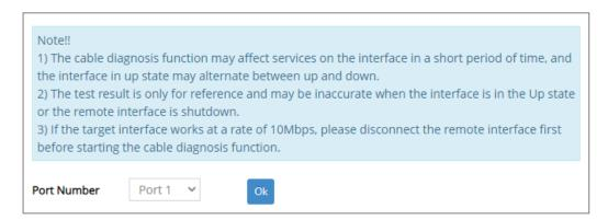
**Port Number:** Select an interface from the drop-down menu to specify which port will be diagnosed. After the selection, click on the **OK** button to run the cable testing. A **Cable Diagnosis Result** section will appear right below **Port Number**.
