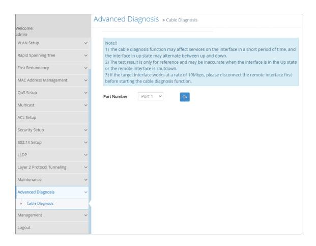
**1. Cable Diagnosis:** Perform Ethernet cable tests on the selected interfaces to enable efficient fault investigation and simplified network troubleshooting.
