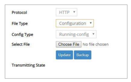
**Config Type:** There are three types of the configuration file: Running-config, Default-config and Start-up-config.
