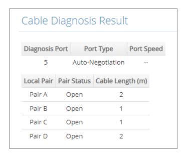
Cable Diagnosis Result: The test result of Cable Diagnosis performed on the target interface.
