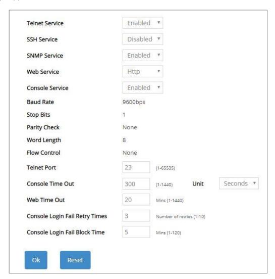
**Telnet Service:** To enable or disable the Telnet Management service.
