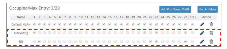
**NOTE:** By default, all ports are member ports of the Default\_VLAN. Before removing the Deafult\_VLAN from the VLAN table, make sure you have correct management VLAN and VLAN mode configurations, otherwise, incorrect configurations may disconnect your management PC to the Managed Switch immediately when you enter the command.
