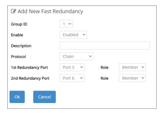
Step 3: Set up the Chain configuration on Switch 3.
