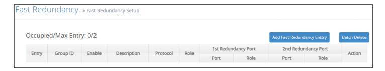
**1-3.** Please refer to each column parameter below, set "Group ID" = 1, "Enable" = Enabled, "Protocol" = Chain, "1st Redundancy Port" = Port 5, "1st Redundancy Port / Role" = Head, & "2nd Redundancy Port" = Port 6, click **OK** when completing the chain configuration for Switch 1.
