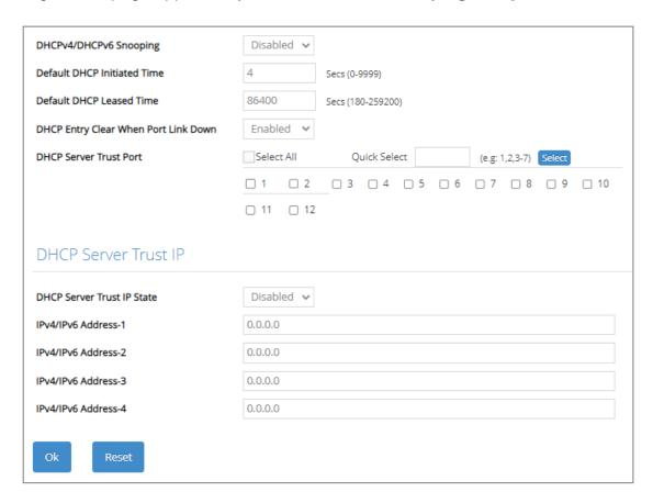
**DHCPv4/DHCPv6 Snooping:** Enable or disable DHCPv4/DHCPv6 Snooping function.
