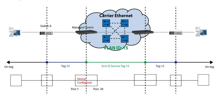
Q-in-Q VLAN Network Diagram
