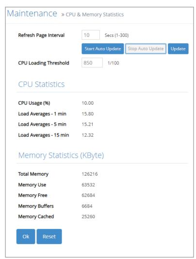
**Refresh Page Interval:** Automatically updates statistics of CPU & Memory at a specified interval in seconds. Please note that the value you assign in this parameter is temporarily used and will not be saved into the configuration file of the Managed Switch. This value will not be applied into the next system boot-up.
