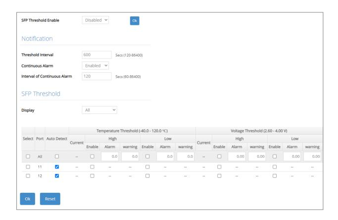
**SFP Threshold Enable:** Globally enable or disable the alarm notification of temperature/current/voltage/TX power/RX power for SFP ports of the Managed Swtich.
