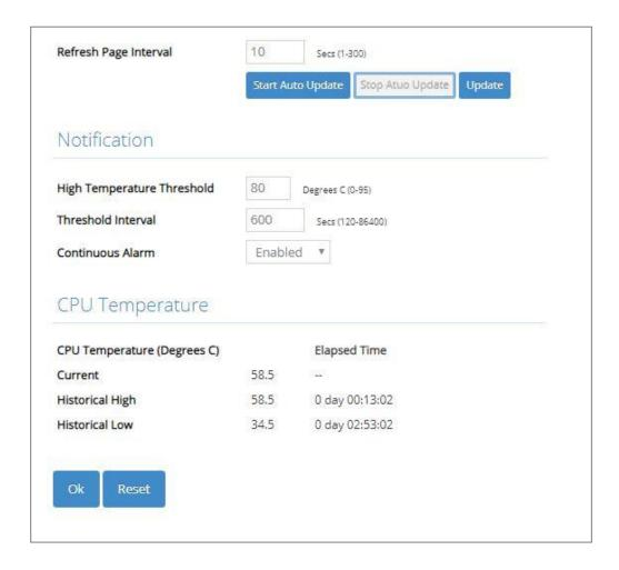
**Refresh Page Interval:** Automatically updates CPU temperature of the system at a specified interval in seconds. Please note that the value you assign in this parameter is temporarily used and will not be saved into the configuration file of the Managed Switch. This value will not be applied into the next system boot-up.
