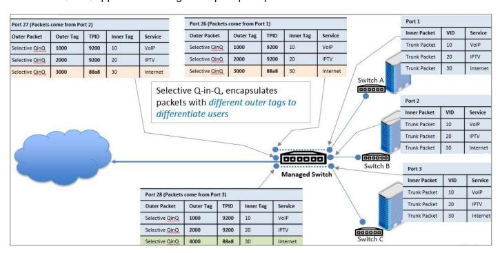
As the above figure shows, three clients are assigned three VLANs that the tag values are 10, 20 & 30 in internet service. VLAN 10 corresponds to VoIP, VLAN 20 corresponds to IPTV and VLAN 30 corresponds to Internet. After the downlink ports enable selective QinQ function that connects Managed Switch to switch A, B & C, the packets will be packed with different external tags according to VLAN ID of service.
