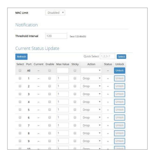
**MAC Limit:** Globally enable the MAC Limit function of the switch. After that, proceed to further port settings as shown below.
