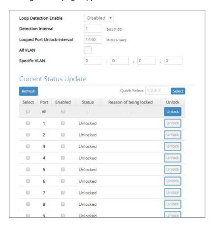
**Loop Detection Enable:** Check to enable the Loop Detection function on a system basis. The default setting is disabled.
