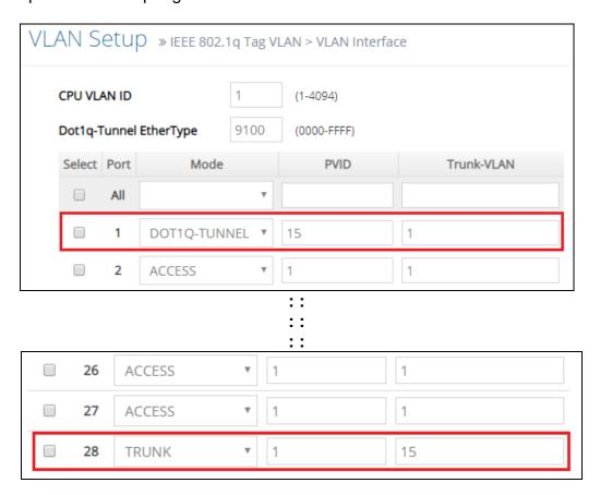
Check the VLAN status. Supposed that Port 1 carries dot1q-tunnel VLAN 15 while Port 28 trunk VLAN 15.
