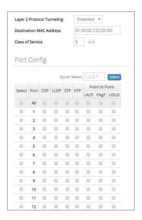
Layer 2 Protocol Tunneling: Enable or disable the Layer 2 Protocol Tunneling fuction globally.
