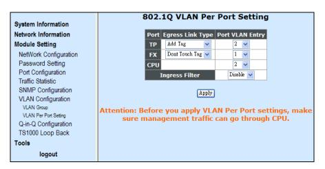
Step 1. Set TP port's Egress Link Type to "Add Tag" and select VLAN Group 2 (330). When Management PC1 sends out a frame, the Converter will remove VLAN tag 330 within a frame. To ensure the link will not be disconnected due to the lack of the appropriate tag, TP port's Egress traffic should be added a tag 330.
