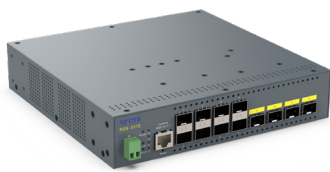
FOS-5112 8-Port 1G Fiber + 4-Port 10G Fiber Managed Switch
