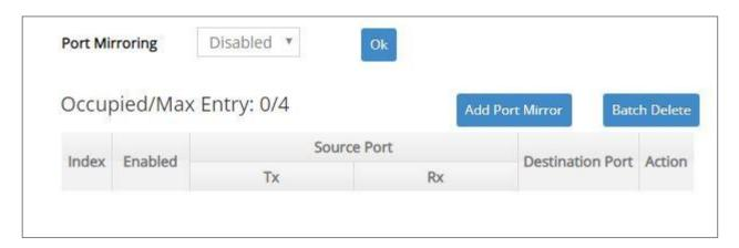
This table will display the overview of each configured port mirroring. Up to 4 sets of port mirroring can be set up.
