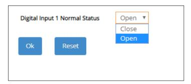
There is one Digital Input Normal Status option shown on the screen page. Normal Status refers to where the contact remains in one state unless actuated. The contact can either be normally open until closed by operation of the switch, or normally closed and opened by the switch action. You may choose either "Open" or "Close" as the normal status of electrical circuit by clicking this pull-down menu.
