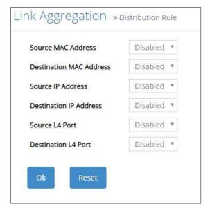
There are six rules offered for you to set up packets according to operations.
