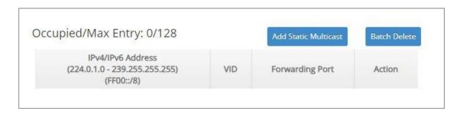
This table will display the overview of each configured static multicast entry. Up to 128 static multicast entries can be created.
