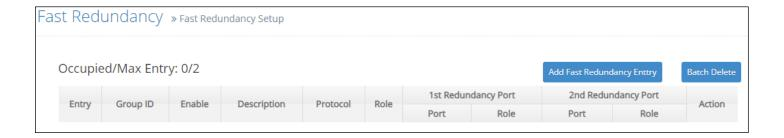
**1-3.** Please refer to each column parameter below, set "Group ID" = 1, "Enable" = Enabled, "Protocol" = Fast Ring v2, "Role" = Master, "1st Redundancy Port" = Port 5 & "2nd redundancy Port" = Port 6, click **OK** when completing the Fast Ring v2 configuration for Switch 1.
