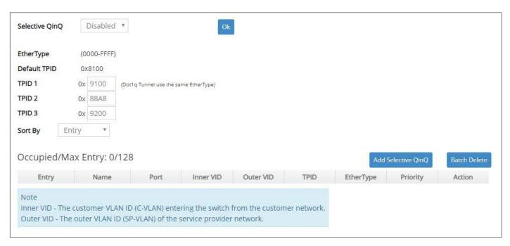
This table will display the overview of each configured Selective Q-in-Q rule. Up to 128 Selective Q-in-Q rules can be set up.
