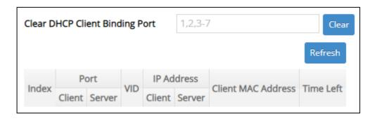
Clear DHCP Client Binding Port: Clear the DHCPv4/DHCPv6 snooping entry. Specify the DHCP client binding port, and click Clear to remove the intended DHCPv4/DHCPv6 snooping entry.
